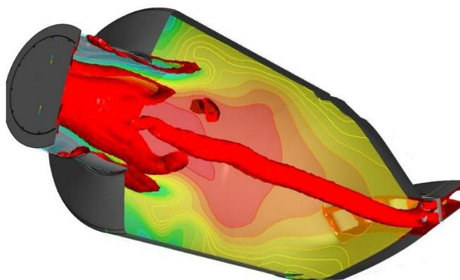
Figure 1. Temperature contours as well as isosurfaces of high vorticity in gas turbine combustor.
